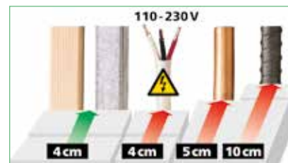
Wood / metal beam Non-ferrous metals (copper etc.) Live electrical cables Ferrous metals (steel etc.)
