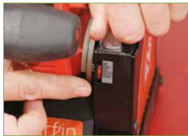
Adjustment of depth with index
