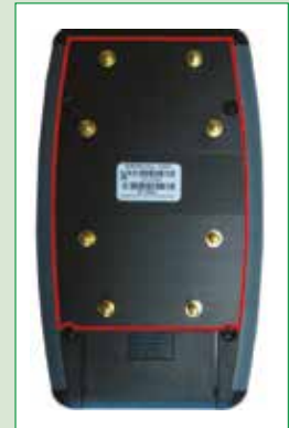
8 spring electrodes forming a very wide measurement area
