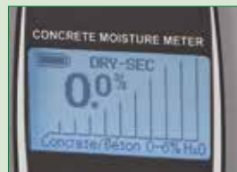
Concrete support scale Beeps at 4.5 %
