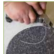
Groove round cuts by removing the rear grooving blade
