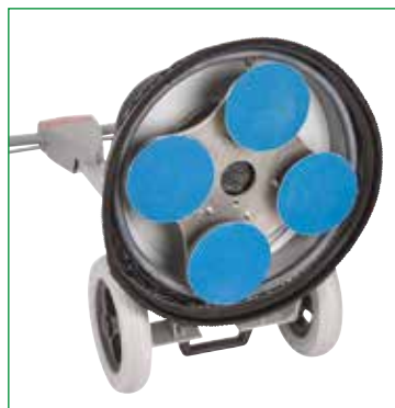
Satellite metal drive disc holder with 4 discs with self-gripping backing. Rotation speed: • Disc holder: 150 rpm • 150 mm disc: 300 rpm
