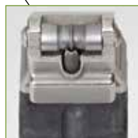
Front grooving blade perfectly centred with regard to the guide wheel
