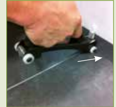
Raising the groover and pushing, you can groove the last cm.
