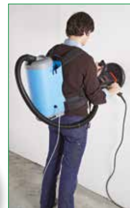
Can be connected to "PBV-225" slow sander for external thermal insulation polystyrene plates.
