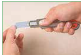
1 Take the used blade from the front end of the cutter.
