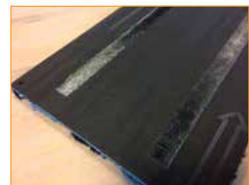
Back tackified adhesive, repositionable.
